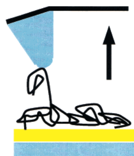
Figure 1. Experimental setup. A polymer is expanded with an AFM tip.
